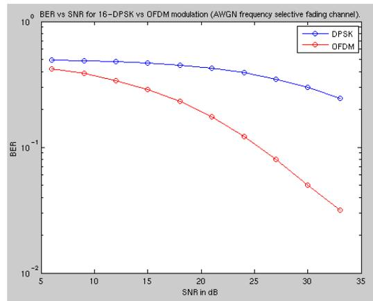
Figure 6.a.: Figure 3.a.: BER vs SNR in a frequency selective channel for 16-DPSK/OFDM (**delay spread=150ns**).
