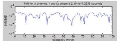
Figure 1.a.: Power Delay Profile (PDP) on an indoor mobile channel      Figure 1.b.: Frequency selective indoor wireless channel
