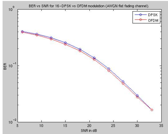
Figure 5: BER vs SNR for a flat fading channel (16-DPSK/OFDM)
