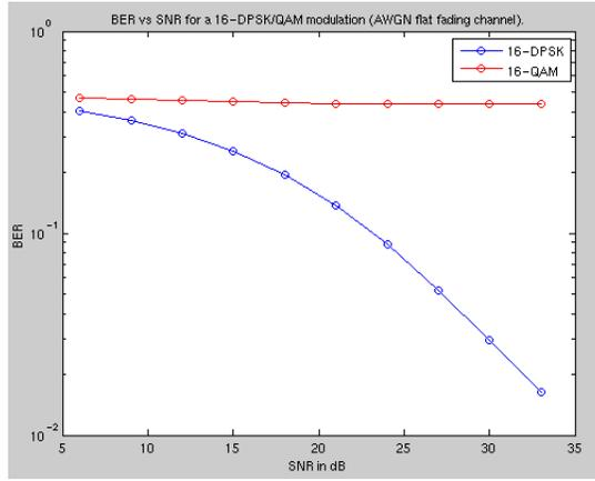
Figure 3.b.: BER vs SNR for an AWGN channel for 16-QAM/DPSK
