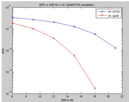
Figure 3.a.: BER vs SNR in an AWGN channel for 16-QAM/DPSK
