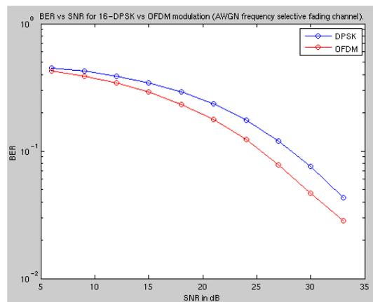
Figure 6.a.: Figure 3.a.: BER vs SNR in a frequency selective channel for 16-DPSK/OFDM (delay spread=15ns).
