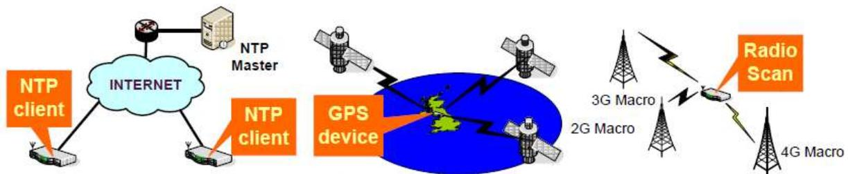
Figure 4: Femtocell current synchronization solutions [11]
