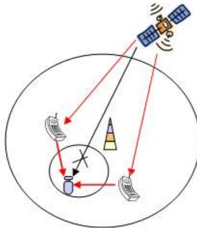
Figure 3: Femtocell 2-D location via mobile sensing
