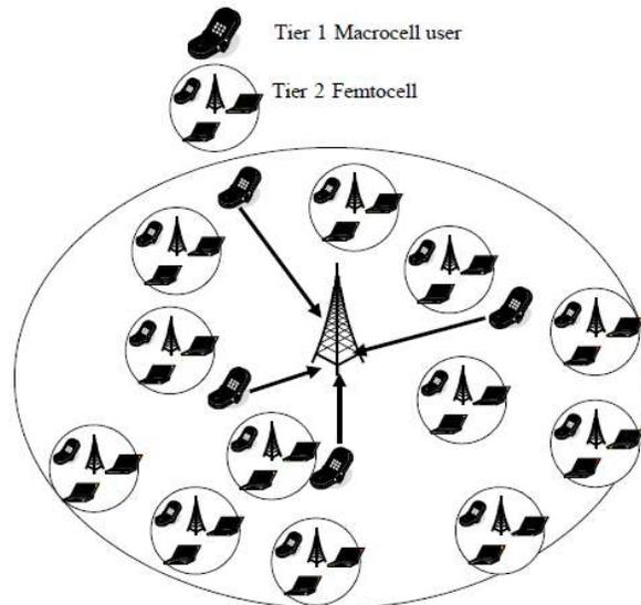
Figure 1: Network architecture of a cellular deployment with femtocells
