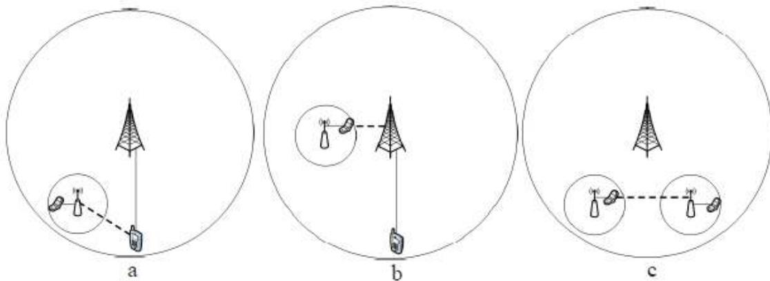
Figure 2: (a) MC user to FC interference, (b) FC user to MC interference, (c) FC to FC interference
