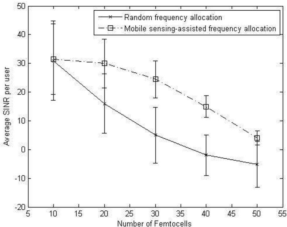
Figure 6: Average SINR [dB] per user for different numbers of femtocells
