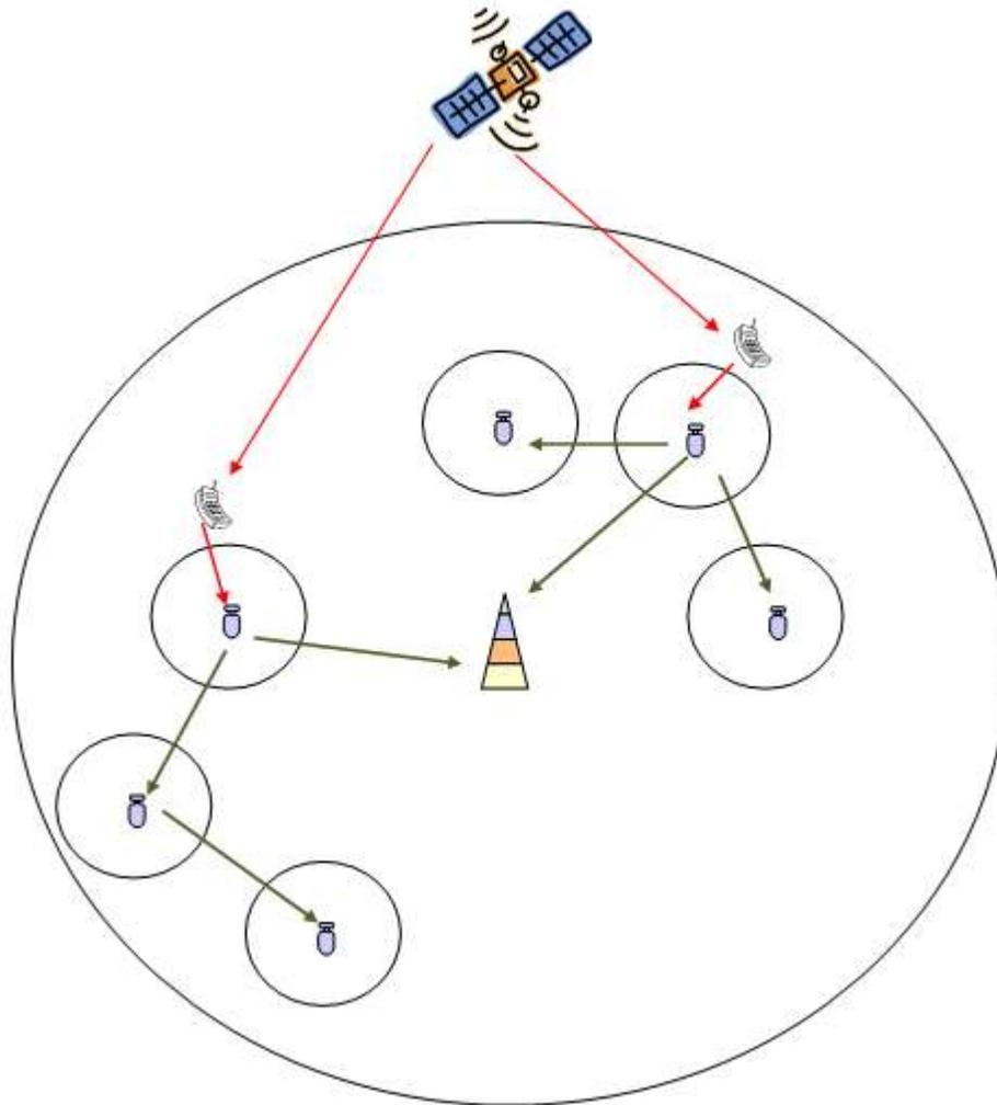
Figure 5: Femtocell deployment as WSN disseminating location information
