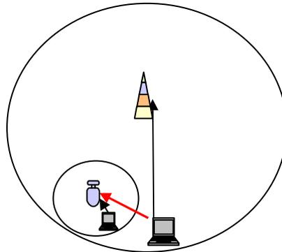
Figure A.1: MC user to FC base station interference
